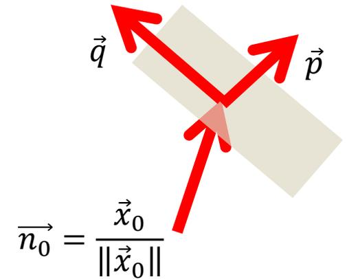
**Astrometric model in local triad (Gaia)**
